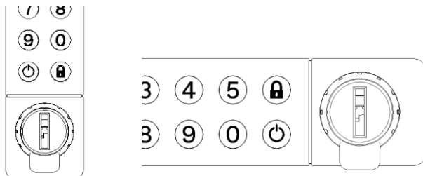
Figure 6. Lock nozzle in close position (Both vertical and horizontal locks (RH&LH))
